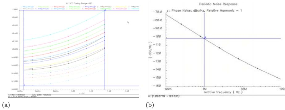
Figure 1: 10GHZ LC VCO(a)Tuning range (b) Phase noise
