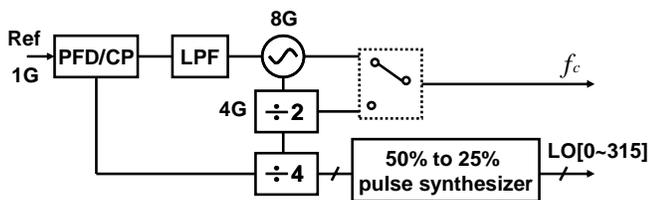
Fig. 1. Block diagram of pulse generator
