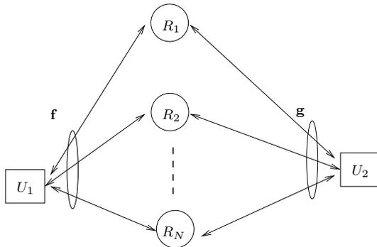
Fig. 1. Two-hop Two-way Parallel Relay Network
