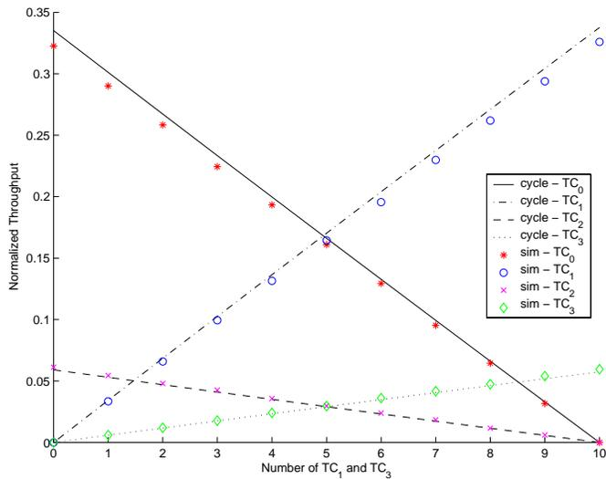
Fig. 1. Analytically calculated and simulated performance of each TC when the number of  $TC_1$  and  $TC_3$  is varied from 0 to 10 (therefore,  $TC_0$  and  $TC_2$  vary from 10 to 0).
