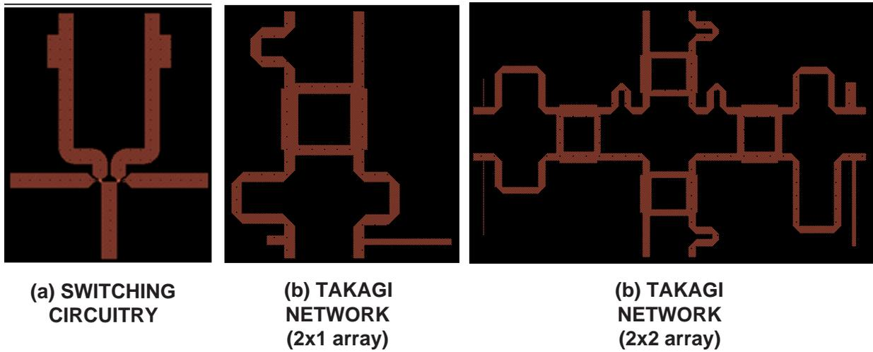
Fig. 1. Microstrip implementation of the decoupling network of the two antennas circular array generated using the Tagaki factorization.
