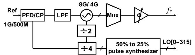
Fig. 2. Revised pulse generator block diagram
