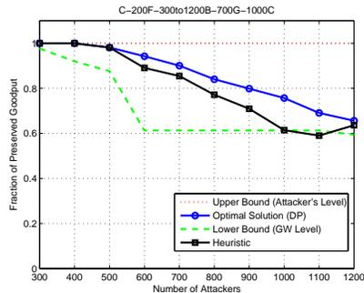
Fig. 4. Code-Red attack based simulation with large number of attackers
