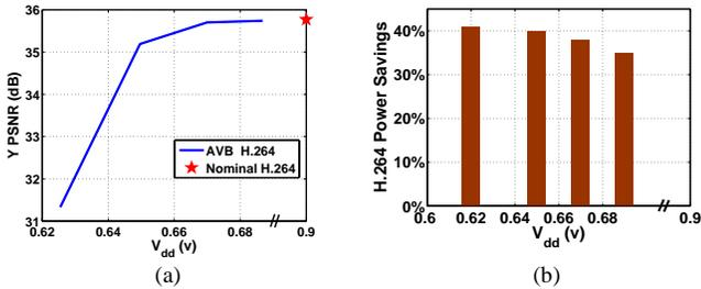
Fig. 2. (a) Effect of AVB combined with filtering on H.264 decoder, (b) expected power saving by utilizing AVB for H.264 and post filtering.
