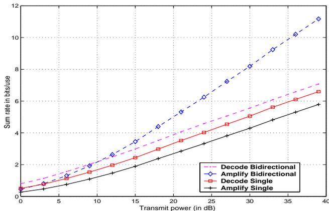
Fig. 3. Average rate of the two way channel in Fig. 1 as a function of transmit power  $P_1 = P_2 = P_R$  for  $N = 2$ .
