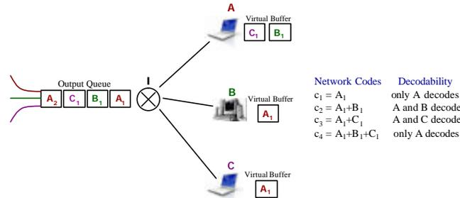
Figure 1: Example of Network Coding for Video (NCV)
