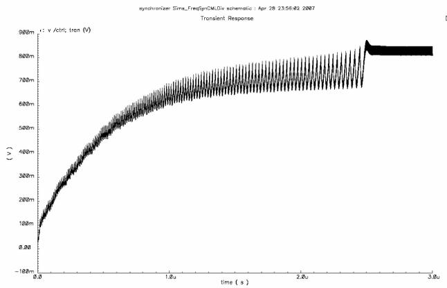
Fig. 3. Control voltage in the PLL
