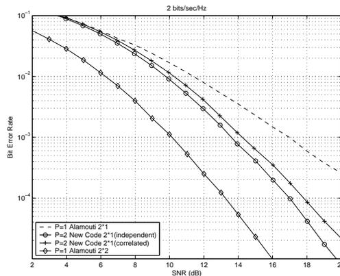
Fig. 1. BER vs. SNR for a remimo; 2 bits/sec/Hz using QPSK.
