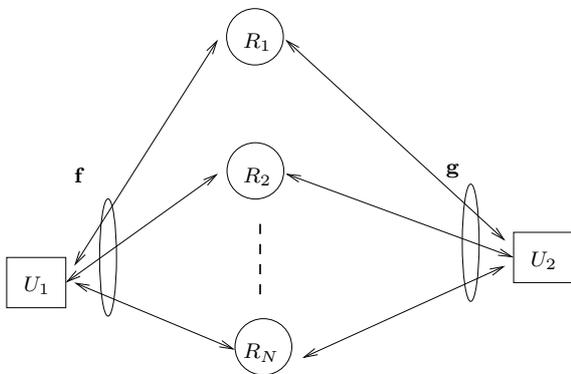
Fig. 1. Two-hop Two-way Parallel Relay Network
