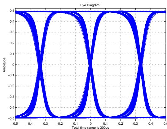
Figure 1: Simulated DFE output eye diagram
