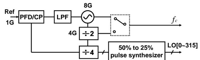
Fig. 1. Block diagram of pulse generator
