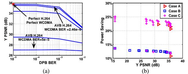
Fig. 4. (a) Utilizing AVB for H.264 and WCDMA, (b) Expected power savings for cases A, B and C.
