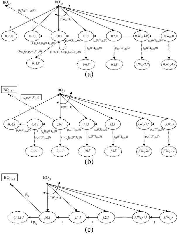
Fig. 1. Parts of the proposed DTMC model for  $N_i=2$ . The combination of these small chains for all  $j, k, l$  constitutes the proposed DTMC model. (a)  $l = 0$ . (b)  $0 < l < QS_i$ . (c)  $l = QS_i$ . Remarks: *i*) the transition probabilities and the states marked with rectangles differ when  $j = r_i - 1$  (as as shown in [2]), *ii*) the limits for  $l'$  follow the rules in [2].
