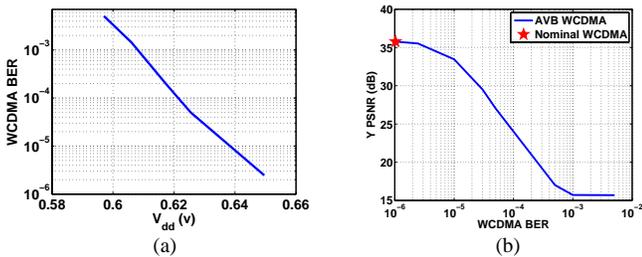
Fig. 3. (a) Effect of aggressive voltage scaling on WCDMA BER, (b) Effect of WCDMA BER on Y PSNR of a perfect H.264 system.
