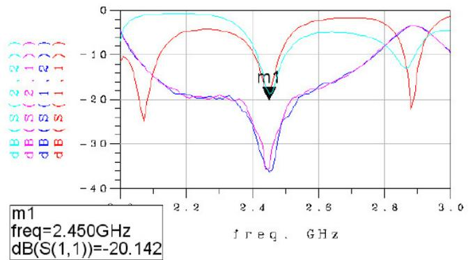
Fig. 3. Simulated scattering parameters at the output of the decoupling network for the two antennas circular array.
