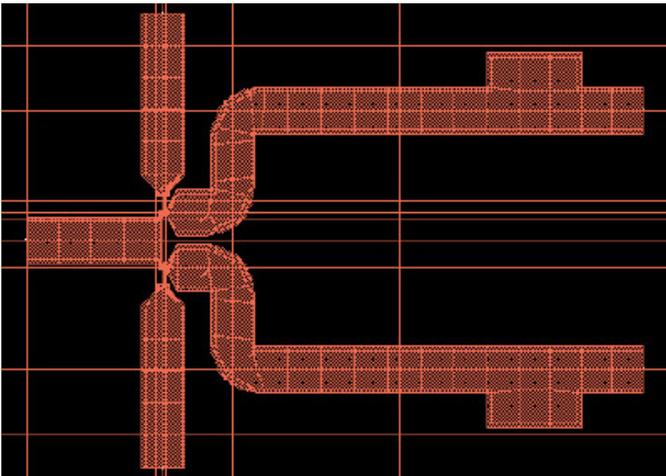
Fig. 2. Microstrip implementation of the switching network with four MEM switches on it.
