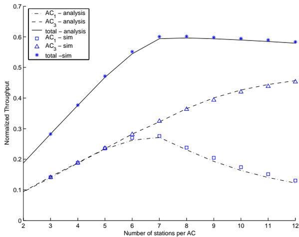
Fig. 3. Normalized throughput of each AC with respect to increasing number of stations when the total offered load per AC is 2 Mbps.
