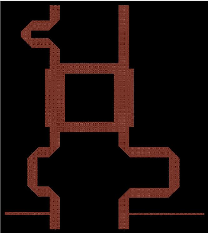
Fig. 1. Microstrip implementation of the decoupling network of the two antennas circular array generated using the Tagaki factorization.
