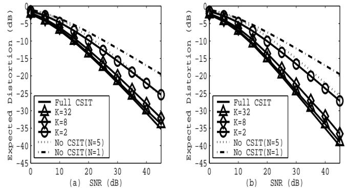
Fig. 1. Expected distortion for a SISO channel with  $b = 1$  (a) Short-term power constraint (b) Long-term power constraint
