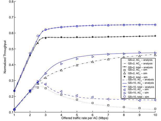
Fig. 2. Normalized throughput of each AC with respect to increasing load at each station.
